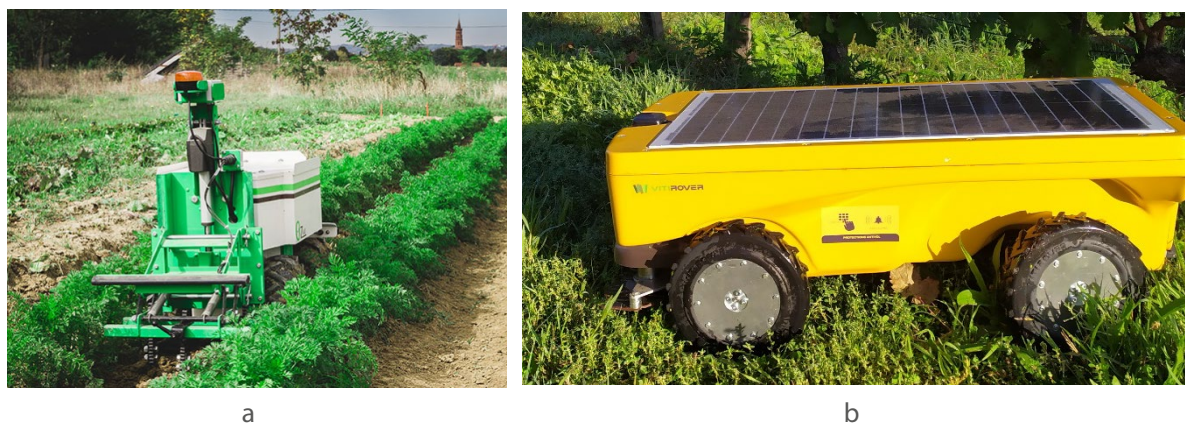
Figure 3.2 Robots for mechanical weeding: courtesy of a) Naio Technologies: Oz b) Vitirover.
