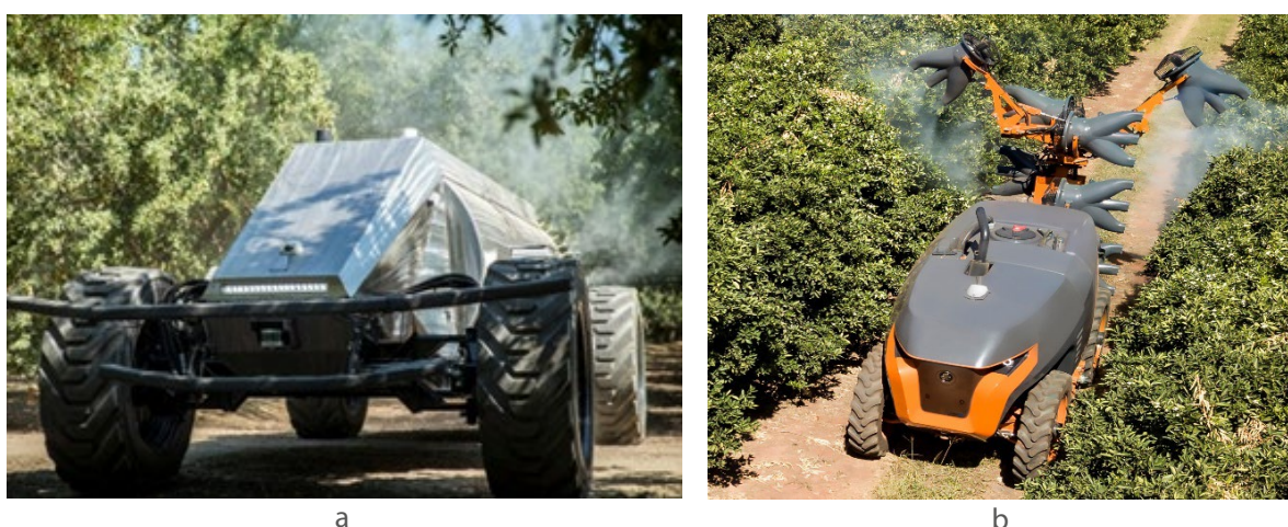
Figure 3.3 Autonomous blast sprayers: a) GUSS (USA); and b) Jacto JAV II, Brazil (with permission).
