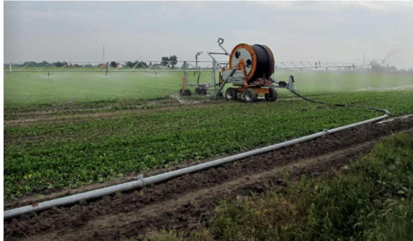
Figure 4.2 Spray boom attached to a reel machine (source Guido Wyseure)
