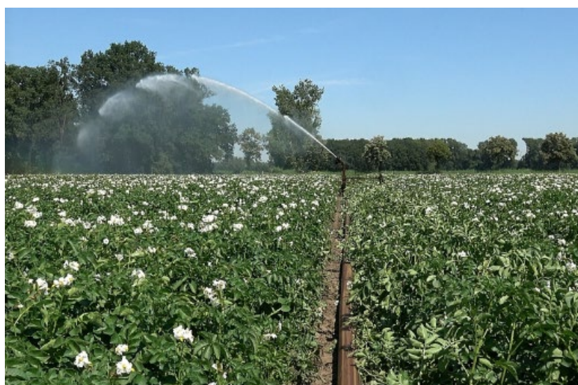
Figure 4.1 Rain gun attached to a reel machine (not in the photo) (source Guido Wyseure)
