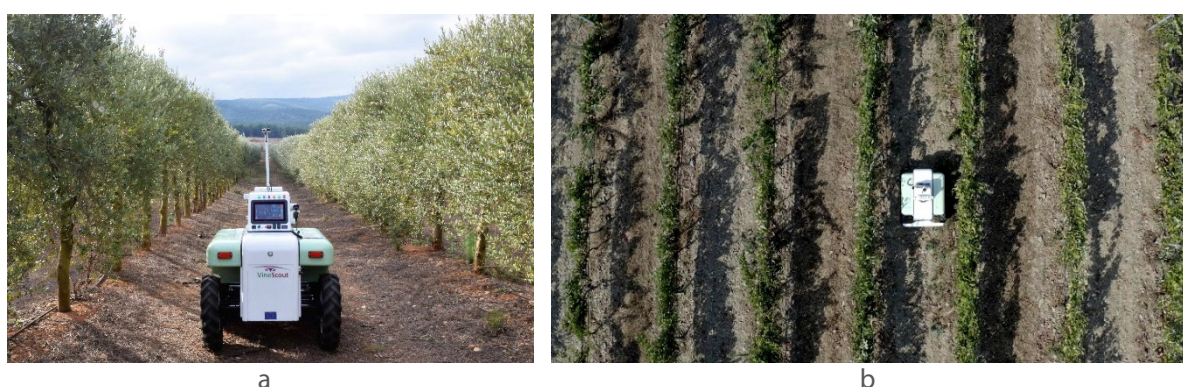
Figure 3.7 VineScout robot for monitoring olive groves (a) and vineyards (b) at high resolution. (source F.Rovira-Más)
